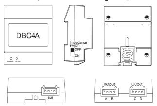
**POWER:** This indicator will light up Red when powered on **IN-USE:** Status indicator. Red light shows the system is in use
