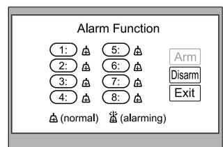
3. **Out-Delay Period:** after you arm the system, you will get into Out Delay Period, monitor will sent out short “Di” every 3 seconds; you will hear a long “Di~” at the end of the Out Delay Period, and the system is gotten into the protecting status. By default, the Out Delay Period is 40 seconds, users must get out off the room within 40 seconds, otherwise the system will treat the user as a invader and sent out the alarm signal.
