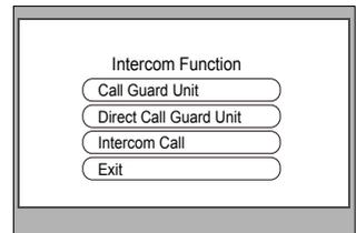
3. **Intercom Call**: you can call the other users in the same network with you. Input the building code and room number by using ▲ / ▼ Button to increase / decrease the value; use ► Button to select next digit; After finish, press **Talk** Button to active the calling, a call message will be sent out, if the system is free, you will heard the feedback rings, you can talk with someone who answers the call. Press ◀ Button to return Intercom Function page.
