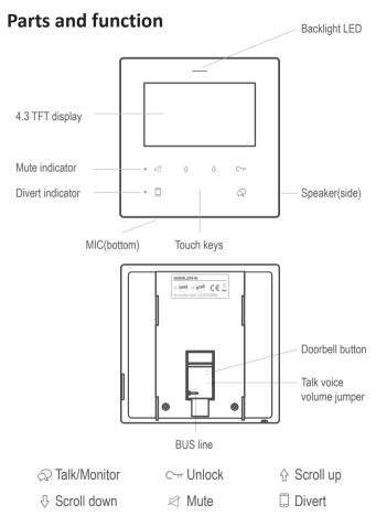
Talk voice volume jumper: the volume of the speaker voice when talk with door station, plug in means high, remove means low.
