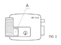
Lock Latch Electric Releas Adjustment (to be performed when the gate is open).
