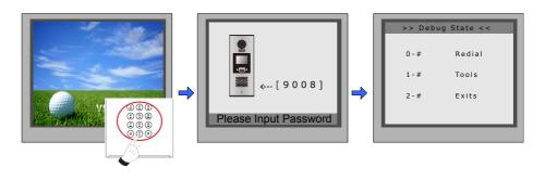
When Door Station is in standby, press '#' key
