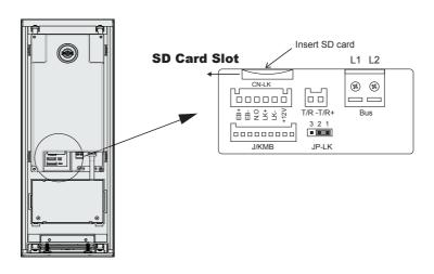
Step 1: Insert the SD card which is contained config files into the SD card slot where is at the back of the door station. Refer to the right diagram.
